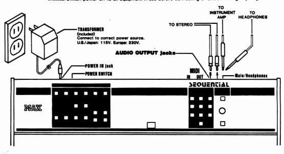
WARNING! Switch power off to all equipment in use before connecting or disconnecting anything
