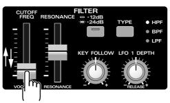
You will hear a characteristic synthesized sound. A combination of changes in [CUTOFF FREQ] and [RES-ONANCE] is one of the most frequently used sound modifications on synthesizers.
