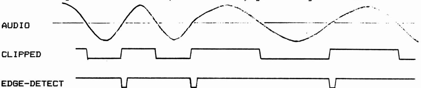
2. The pulse generated by positive zero-crossings of the waveform is about 6 usec. wide and the pulses are either 1/4800 of a second or 1/2400 of a second apart.
