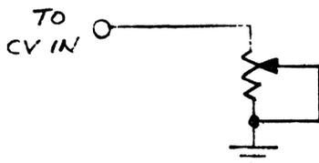
FIG. 3 - FOOTPEDAL WIRING DIAGRAM
