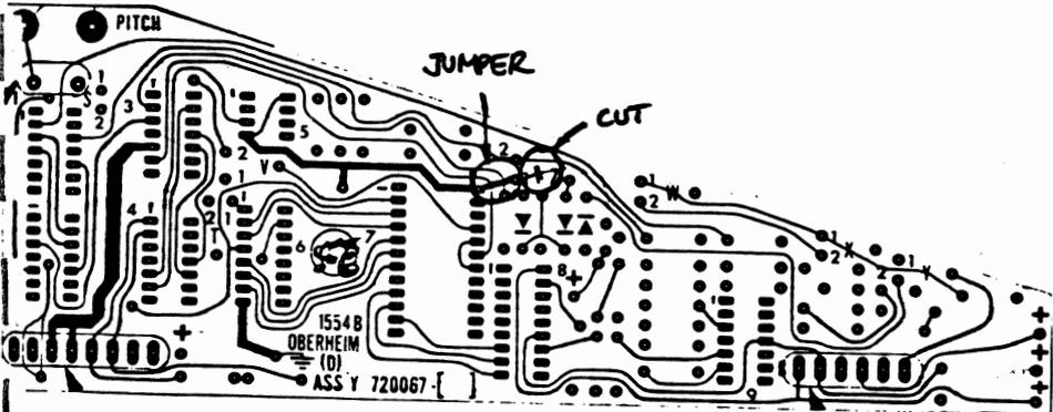
PC 1563B/1564B: 1) CUT TRACE FROM Z1 TO COLLECTOR OF Q1
