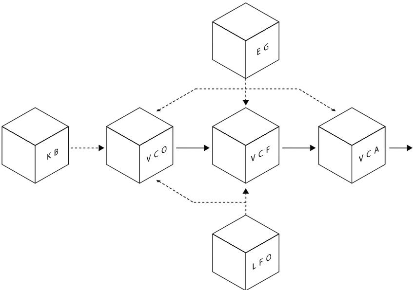
In this diagram of the Werkstatt modules, the solid lines represent audio signals, and the dotted lines represent control signals. The definitions and functions of each module are described in the Werkstatt Features and Controls section.
