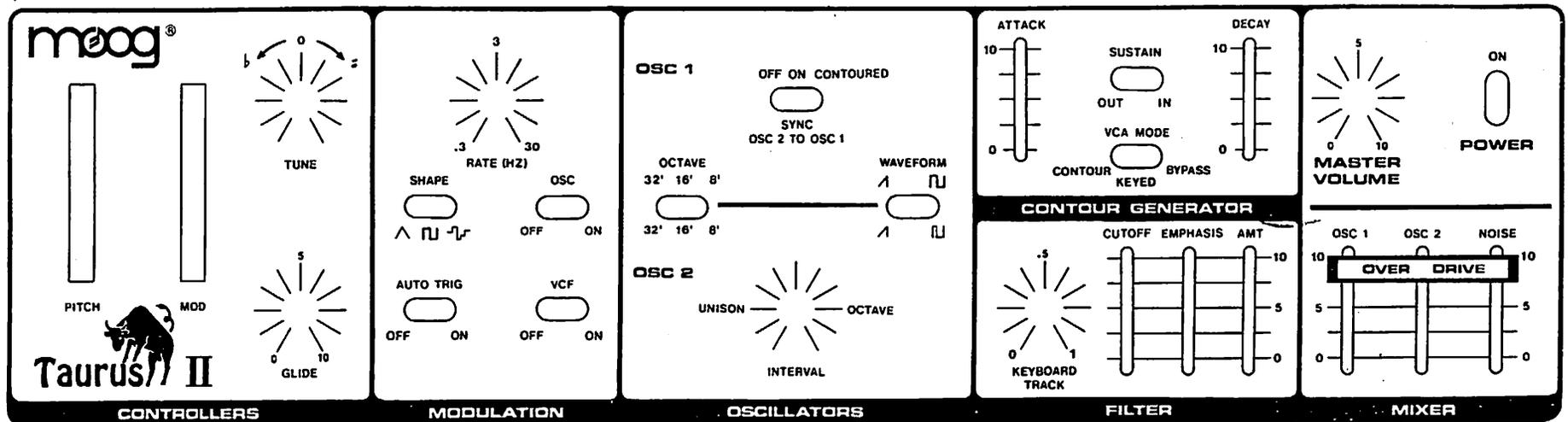
Taurus II sound charts are line drawings of the instrument's front panel. Positions for placing toggle switches, rotary controls and sliders are indicated by dots.
