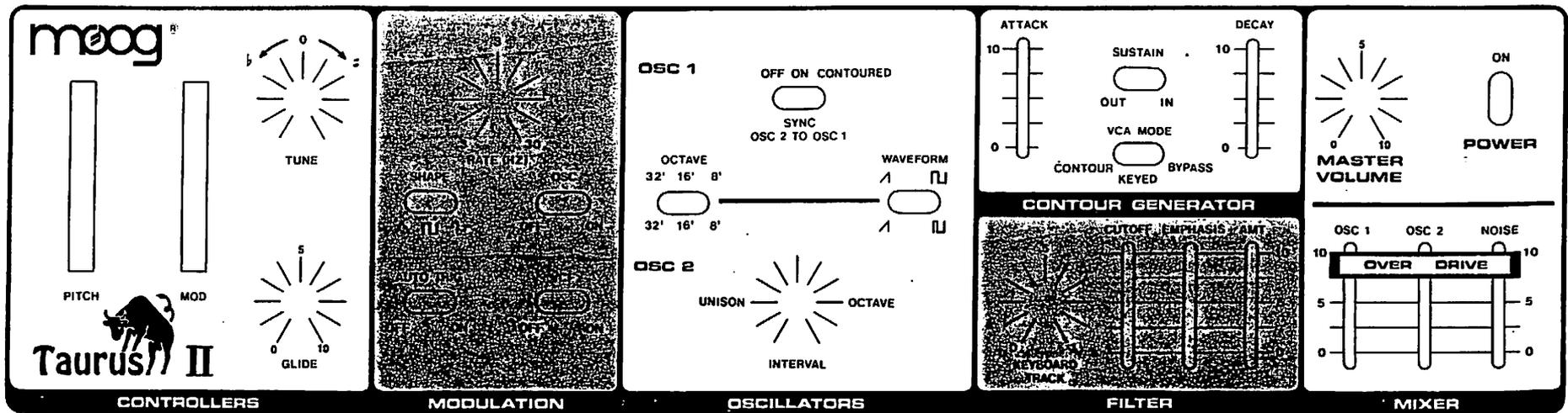
The shading on the above diagram indicates the modulation and filter portions of Taurus II.
