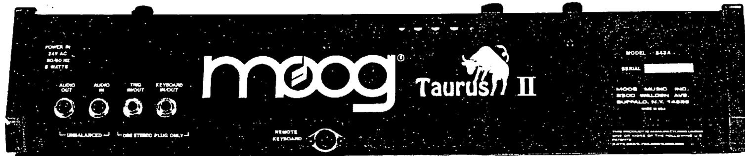
Taurus II has a number of connectors on the rear panel which can be used to interface Taurus II with synthesizers, sequencers and other instruments which are voltage controlled.
