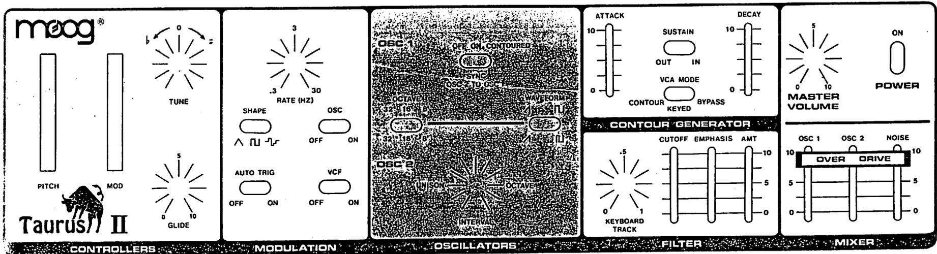
The shading on the above panel shows the location of the audio generator portion of Taurus II.
