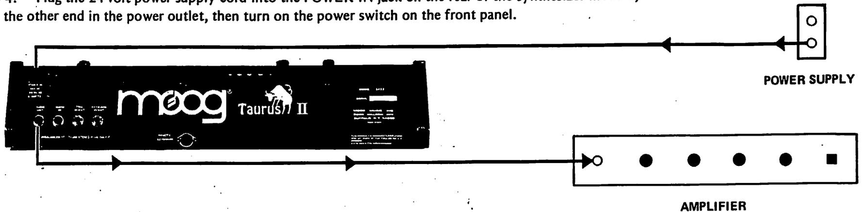
Step 5: Using a 1/4" jack audio cord, connect the AUDIO OUT on the rear of the Taurus II to your amplifier or monitoring system.
