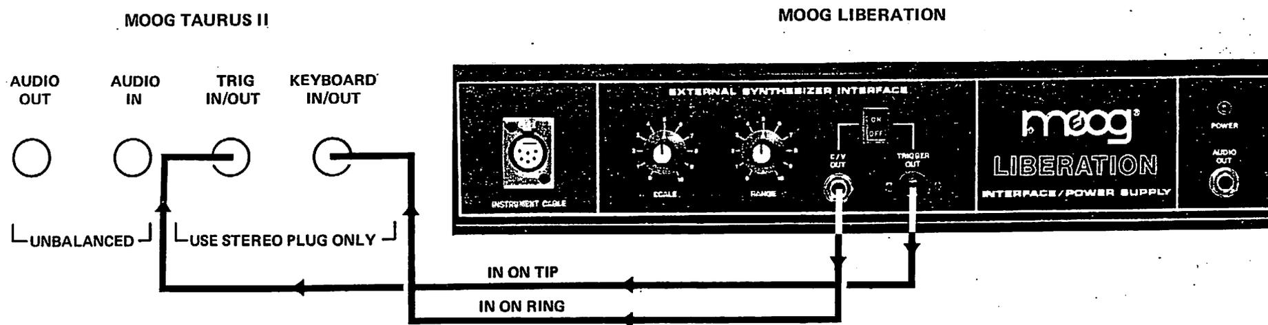
The Liberation's control voltage output must be scaled and ranged. Scaling makes sure intervals are correct on both instruments and ranging ensures unisons are correct. The proper procedure is as follows:
