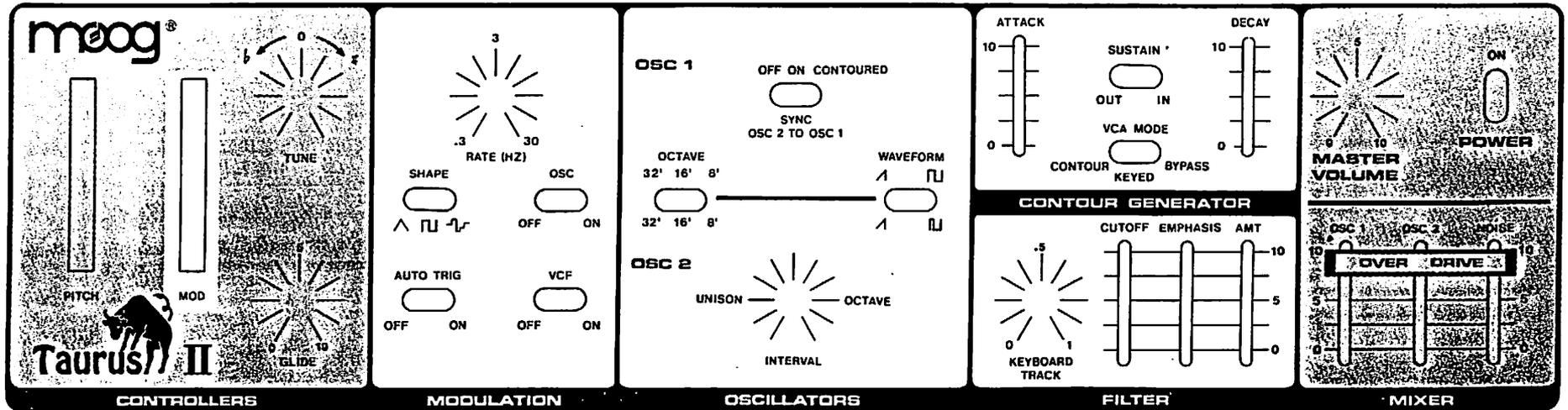
The shading on the above diagram shows the locations of the controllers on Taurus II.
