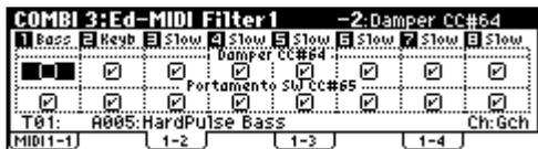
If a check box is checked, the corresponding MIDI data can be sent and received. If “Status” is INT, movements of the X50’s controllers or incoming MIDI data will apply an effect for the program of that timbre. (Effect Dynamic Modulation functionality is not affected by these settings.) If the “Status” is EXT or EX2, movements of the X50’s controllers will transmit MIDI data on the channel of that timbre. MIDI transmit/receive settings for the entire X50 are made in “MIDI Filter” (GLOBAL 1).
