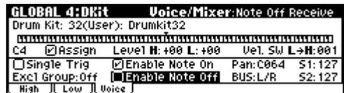
4. For each key, set the Enable Note Off Receive parameter as desired.
