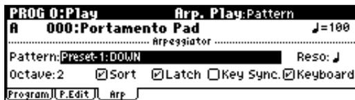
2. Use the ClickPoint [◀][▶][▲][▼] to choose "Pattern," and use the [VALUE] dial or the [INC][DEC] buttons to select an arpeggio pattern. To select a user arpeggio pattern, you can also use numeric buttons [0]-[9] to enter a pattern number and then press the [ENTER] button.
