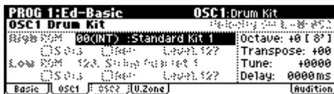
5. Specify the basic pitch of the oscillator. For a drum kit, set “Octave” to +0 [8].
