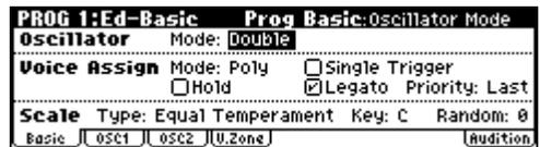
Single Programs have one oscillator, and Double Programs have two oscillators. Each oscillator includes a complete synthesis voice, with velocity-switched Multisamples, dual filters, EGs, LFOs, and so on.
