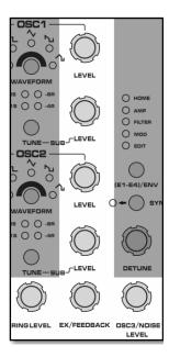
**EXT/Feedback:** [0...127] Determines "External Audio Level" or "Feedback Amount". You can use only one function regarding the connection of external TRS jack.
