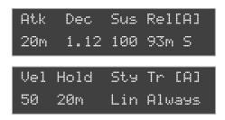
**loop:** when [release = 0] the loop function is enabled this means that the envelope will continuously switch back to the beginning of the attack stage after finishing the decay cycle.
