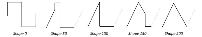
**StpSqr** is a kind of square wave with double steps while the Pulse Width parameter only affects one part. However, you can get a virtual PWM on the second part with modulating Shape:
