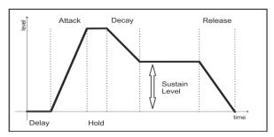
The **Hold** stage freezes the envelope signal level after the attack stage that can be used for increasing punch in percussive sounds with fast attack and decay. Filter and Mod envelopes have 6 stages, but the Amp envelope has 5 stages (without delay).
