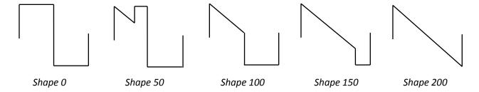
Besides **Shape** value the **pulse width** setting can also change the Square wave independently which results in creating of more complex and unpredictable waveforms with rich harmonics. Don't forget to tweak the shape and pw to find the sweet spots. You can modulate the shape and pw at the same time too.
