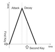
**LFO2SH:** Forces the envelope to start from the beginning of the attack stage at each clock cycle of LFO2 when S&H is selected as waveform.
