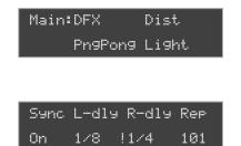
**Sync:** [On, Off] when on, DFX delay time can be controlled with note values between 1/2 and 1/32 notes. The rate is then dependent on the tempo setting. If the selected synced rate for Px is more than the maximum delay length of the algorithm, it will be marked with an exclamation point "!" on the screen showing that you must switch to a shorter delay time. (Soft Knob E1)
