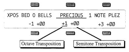
Each track can have its pitch transposed (raised or lowered) by octaves and semitones within an eight octave range. The transpose setting affects both the pitch played by Local VFX voices and the key number transmitted via MIDI.
