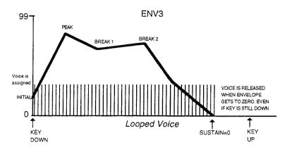
For a sustaining wave, when the Envelope Mode is set to Finish:
