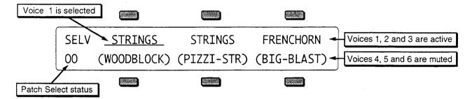
The six locations on the screen represent the six voices which are available within the program. For each voice the display shows the name of the wave that the voice is assigned to play, and the mute status of the voice in the current patch. When you press the soft button above or below one of these voices, it becomes <u>underlined</u>, indicating that it is the currently selected voice, the one that will be affected by any editing you do.
