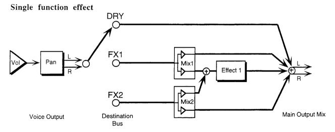
The above illustration shows the effects busses and the output mixing. Every voice is assigned to one of the three stereo busses, which go around or through the effects processing. The heavy lines are stereo paths.
