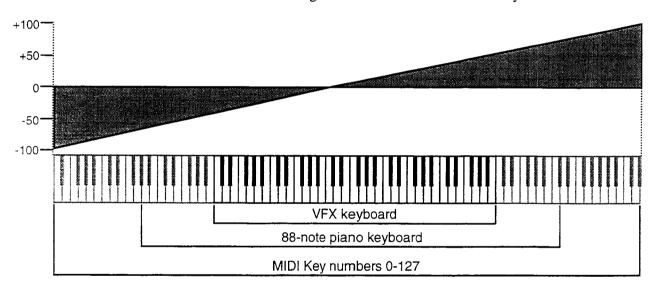
As the above illustration shows, the effect of KEYBD as a modulator goes negative as well as positive. The effect of KEYBD is to reduce the Level on notes below the break point (Middle C), and increase levels above that point. Negative Modulation depths will do the opposite.
