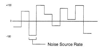
The Noise Source Rate defines how frequently the level will change. Low values will cause it to change very slowly; with high values the level will change quickly.
