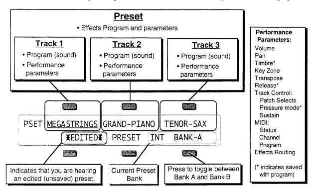
Whenever the *Presets* LED is lit, this indicates that the VFX is in Preset mode, and the 10 Bank buttons beneath the display will now select presets (rather than selecting Program Bank pages, as they do when the *Sounds* LED is lit).
