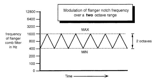
If the settings are modulated, then both the fixed frequency of the notch and/or range of frequencies in the sweep can be affected. Modulated sweeps can be implemented by setting MIN and MAX to the same value (or close together) and modulating them by the same amount. Manual sweeps can be implemented by selecting a modulation source such as the mod wheel.
