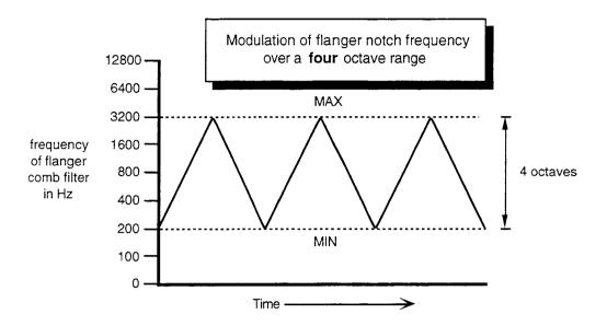
These illustrations show how the relationship between the MIN and MAX settings will determine the frequency range and *apparent* rate of the flanger sweep. The actual rate at which the sweep changes from MIN to MAX is constant, so if the range is narrow, the apparent or perceived rate will be faster.
