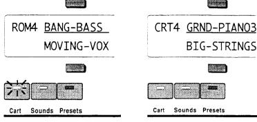
When the Sounds LED is on and the Cart LED is flashing, the VFX is playing programs from its internal ROM memory. The upper left corner of the display shows ROM plus the bank number (0-9).
