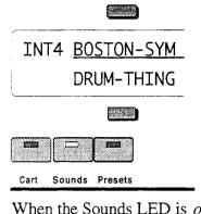
When the Sounds LED is on and the Cart LED is off, the VFX is playing programs from its internal RAM memory. The upper left corner of the display shows INT plus the bank number (0-9).
