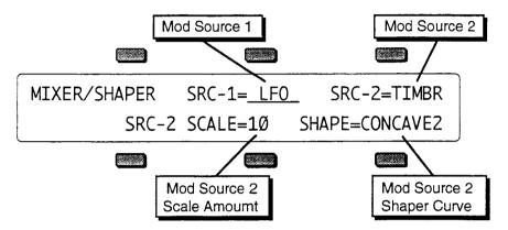
The two controls on the top line of the display select the two modulators which will be mixed together, SRC-1 and SRC-2. On the lower line of the display are two parameters for shaping the level and response of SRC-2. Internally, the Mixer/Shaper works like this:
