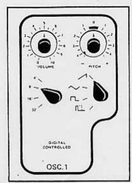
The Oscillator 1 generates the source or raw sound which will be modified by the other controls on the synthesizer. This is your primary oscillator so use it to tune to a-440 or to the other instruments in the group.
