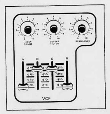
The envelope shape, range, cut-off, and resonance work with one another to produce vastly different effects from a single source, and virtually unlimited effects from all combinations of sources.
