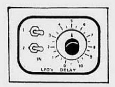
Then, the amount of delay before the activated LFO's start to take effect is determined by the LFO Delay Control on the right.
