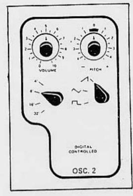
The Oscillator 2 contains essentially the same specifications and features as Oscillator 1 except for two differences: (1) the range of Oscillator 2 is an octave and a half and (2) there is no variable pulse wave form. This oscillator can be used for unison tunings or parallel intervals with Oscillator 1 such as 3rds, 4ths, 5ths, 7ths. If a phasing effect is desired put Oscillator 2 slightly out of tune with Oscillator 1.
