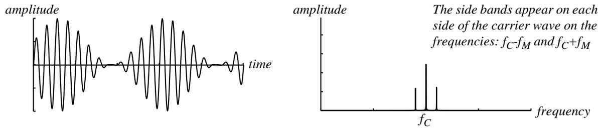
**Fig 3. Amplitude Modulation**
