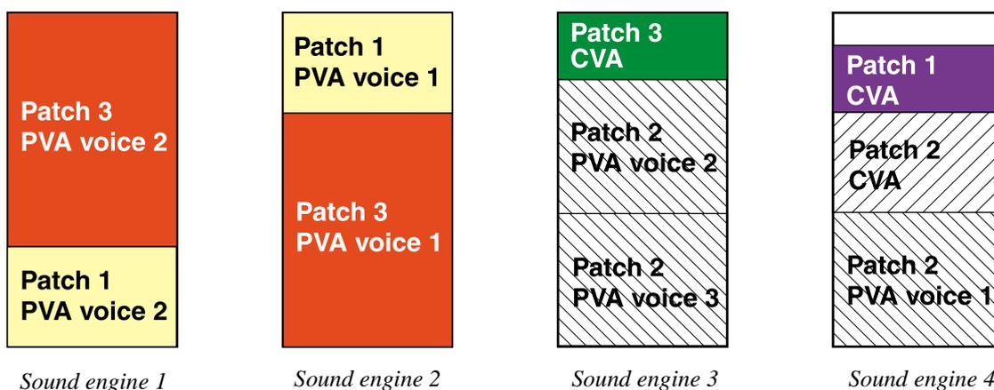
In a multi-patch situation the distribution of Sound engine resources is made evenly between the patches in the selected slots, and with the aim to use the Sound engines in the most optimal way. The different Voice Areas of the patches could end up anywhere in the Sound engine(s), but always in the most optimal combination.
