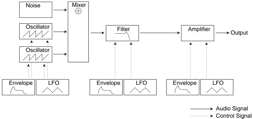
Note that the horizontal lines indicate the way the sound travels. The vertical lines indicate control signals. The envelopes for example only *modulate* (control) the oscillator, filter and amplifiers, they do not affect the sound directly.
