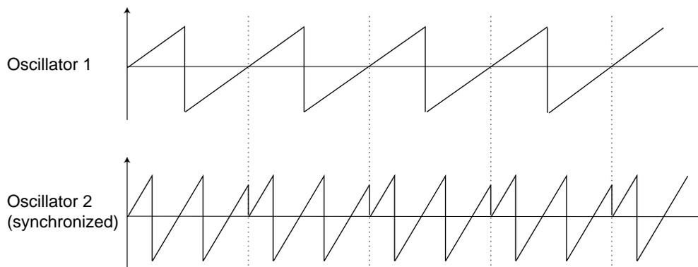
When sync is applied, the basic pitch of Oscillator 2 is locked to that of Oscillator 1. If you change the pitch of Oscillator 1 you will affect the basic pitch of both oscillators. Furthermore, when you vary the
