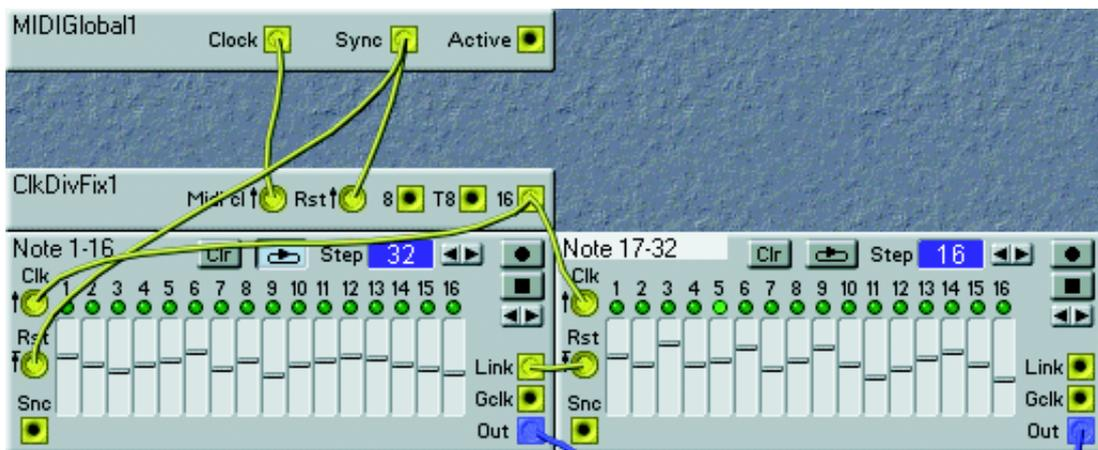
The loop mode of the second sequencer in this example is off. When the signal from the first sequencer's Link output resets the second sequencer, the second sequencer will start sequencing its 16 steps. The first sequencer, which was set to 32 steps, will be inactive during these 16 steps. When the second sequencer has performed its 16 steps, the first sequencer restarts again.
