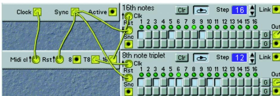
In this example, the clock is taken from the MIDI global module, at 24 pulses for each quarter note. It is divided with the fixed divider module with two different division ratios, 16 and T8. The divider module is reset by the logic signal from the Sync output on the MIDI global module. This reset signal is also used on the two sequencer modules. The Global Sync function which is found in the Synth Setting menu determines the rate of the pulse at the Sync output.
