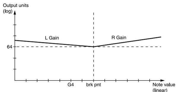
*Figure 2. Velocity sensitivity is increased, which means that note values affect the output according to the Gains, but the offset has now become a velocity range. The velocity range is controlled with the Vel Sens knob.*
