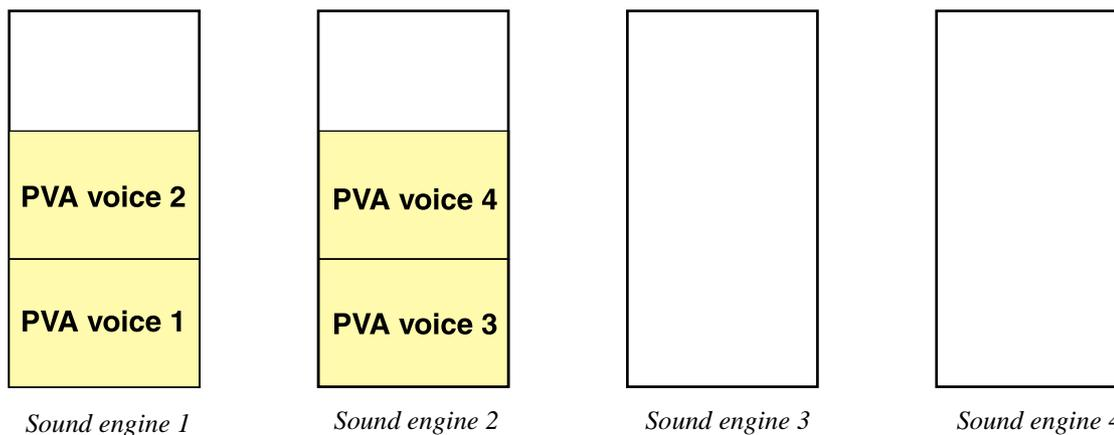
This comparison shows one benefit of using both voice areas of the patch, the Poly Voice Area and the Common Voice Area. In the first example our patch occupied only one Sound engine, and in the second example the patch required two Sound engines, even though the voice amount was the same in both cases.
