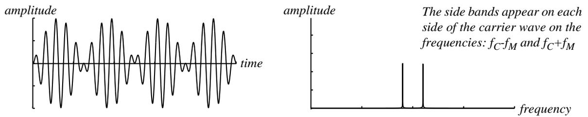
**Fig 3. Ring Modulation**
