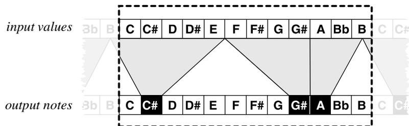
*Here we have activated the Cont function. As you can see, the input signal will be quantized to the selected notes in equal sections, per octave, across the selected range.*
