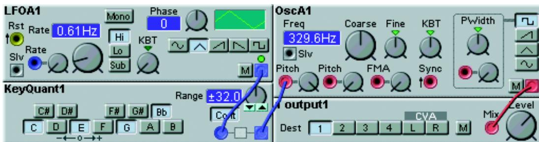
LFO A is set to generate a triangle wave, since this signal has linear, symmetrical ramps. This guarantees even change of control values over time. We have pressed four Note buttons and selected a Range of +/- 32 semitones on the KeyQuant module. The output signal from the KeyQuant module is routed to one of the Pitch inputs of the Osc A module. The Pitch mod attenuator of the Osc A module is set to 127 to ensure correct semitone intervals.
