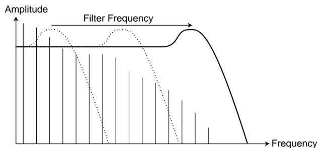
Changing the cutoff frequency is often referred to as “sweeping the filter”. This is probably one of the most important ways of shaping the timbre of a synthesizer sound. By using an envelope you can for example have a high cutoff at the beginning of a sound which is then gradually lowered (the filter “closes” as the sound decays). This would emulate the way most plucked string sound (piano, guitar etc.) behave; the amplitude of the harmonics decreases as the sound decays.
