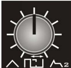
Two independent pulse width modulation controls (PWM), one for each VCO. This allows modulation of the square wave 'duty cycle'. Once again, don't worry about this technically, just enjoy the effect!
