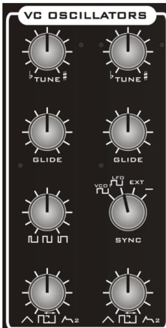
The voltage controlled oscillators (VCOs 1 and 2) produce the raw audio waveform usually used as the initial source for sound creation. They provide cyclic audio waveforms that can be pitched. VCOs usually receive treatment from the VCF to turn their basic tones into pleasant sounds.
