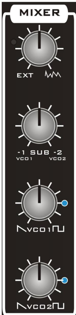
The mixer is used to bring various audio source signals together for filtering. There are four mixer controls. In all cases, centre is zero volume, or turn to the left or right to select either of two sound sources.
