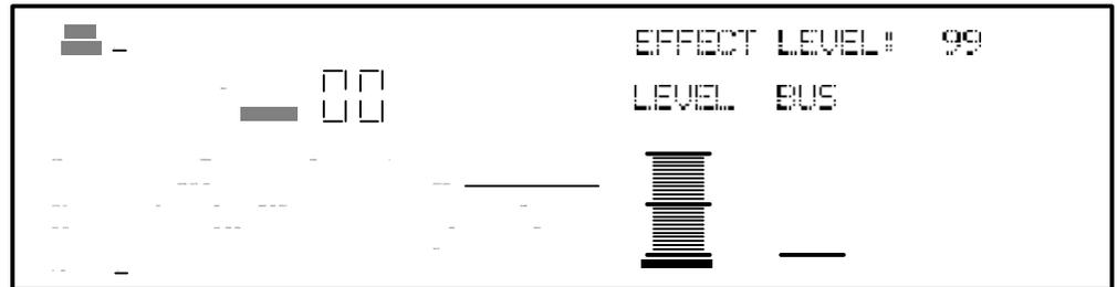
Turn Quad Knob [1] to adjust the effect send level of the selected Sound (1—4).
