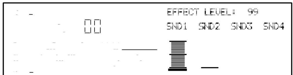
*Note: If a Sound is not enabled in a Program, its title will be shown in lowercase (“snd4”), and adjust its controls will have no effect on the Sound until the Sound is enabled. To enable a Sound, hold down its respective Quad Button (i.e., [3] for Sound #3) and press VALUE [ ].*
