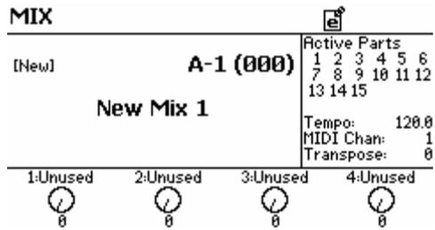
Mix mode is a multitimbral mode that allows you to load up to 16 programs in order to create splits, layer sounds, and set up programs on separate channels for use with an external sequencer. Each program in a mix is stored under its own “part” and the active parts are listed on the upper right corner of the screen. The active part number is highlighted whenever that part is being triggered using the keyboard or an external sequencer.
