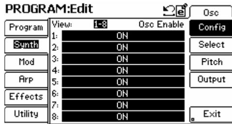
The Synth/Osc/Config screen provides a convenient overview showing how many of the commonly used parameters in the Drum Synthesis submenus are configured.
