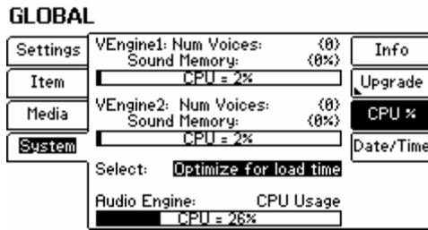
This page is designed to let you know how much of your Fusion’s resources are being used. There are three bars on this screen—the “VEngine1” and “VEngine2” are your “Voice Engines” that are responsible for all synthesis that takes place on the Fusion. The “Audio Engine” bar monitors the processor that handles all recording and playback that takes place on the Fusion’s multitrack recorder.
