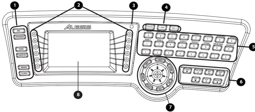
**1. Mode Selection Buttons** (Mix, Program, Song, Sampler, Mixer and Global): These buttons select the main modes of the Fusion.
