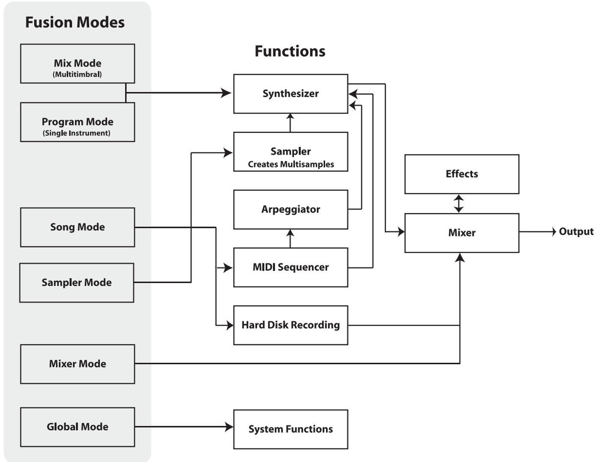
The Fusion is packed with a ton of features and it can be easy to be overwhelmed by it all. Let's take a moment to explain how all the different parts interact with one another.
