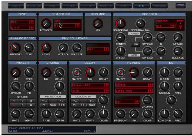
For a full description of any parameter, simply manoeuvre the mouse pointer over it, and take a look at the Information Bar along the bottom of VirusControl.
