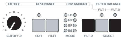
Before we get started with our next experiment, deactivate SATURATION, set the ENV AMOUNT of the filter envelope to zero and set Cutoff 2 to the center position (12 o'clock) so that Filter-2 always has the same cutoff frequency as Filter-
