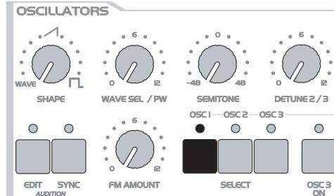
You can definitely see why this waveshape bears the name “sawtooth.” Press and hold a key and slowly turn the pot clockwise. You should be able to hear how the tone becomes increasingly more hollow-sounding. You might say this effect thins the sound out, but in any case, the entire tonal spectrum is affected by an equal measure, which is an audio result filters are unable to achieve.
