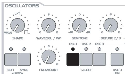
To come up with a fatter sound, you should also dial in the second oscillator (set OSC BALANCE to the center position) and use DETUNE to do just that to its pitch (relative to the first oscillator).
