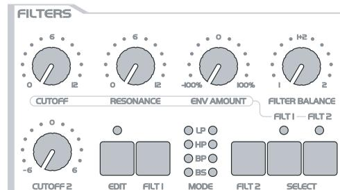
Locate the Cutoff pot (not to be confused with Cutoff 2!) in the section labeled FILTERS, directly above the section labeled AMPLIFIER. Rotate the pot to the left and right and note how the sound becomes muddier and clearer in response to the direction in which you turn the pot. (To ensure this effect and the following aural experiments are most pronounced, adjust the amplifier envelope so that the VIRUS generates a constant level while you hold a key down).
