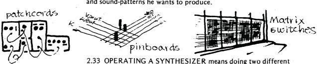
2.33 OPERATING A SYNTHESIZER means doing two different things: one is CONNECTING to each other the devices to be used, or "setting up the patch" as it is called, and the other is SETTING UP, ADJUSTING, AND USING the controls on the devices in the patch.
