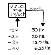
2.212 It is important to remember that VOLTAGE CONTROL is an extension of manual control; in theory anything you can do with a voltage you should be able to do with a knob, manually. IN FACT, your hands cannot move fast enough, or accurately enough, to come within miles of what a voltage signal can do with a voltage-controlled device.
