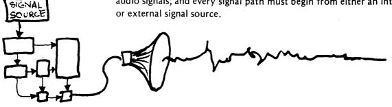
2.3311 Any signal from any device in a synthesizer may be fed directly to an external amplifier or recorder. More commonly it will be routed through other devices before reaching the synthesizer's main output channels. Several signals may be combined in a mixer, or one signal may be split to follow two different paths, which, modifying it in different ways, may later recombine.
